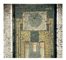
Salt and dirt can damage the sensor of an air mass sensor – or at least distort the measurements, which in turn can have an effect on the EGR.
