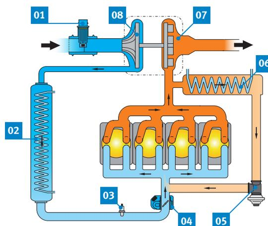
Fig. 2: Schematic diagram of cooled exhaust gas recirculation
