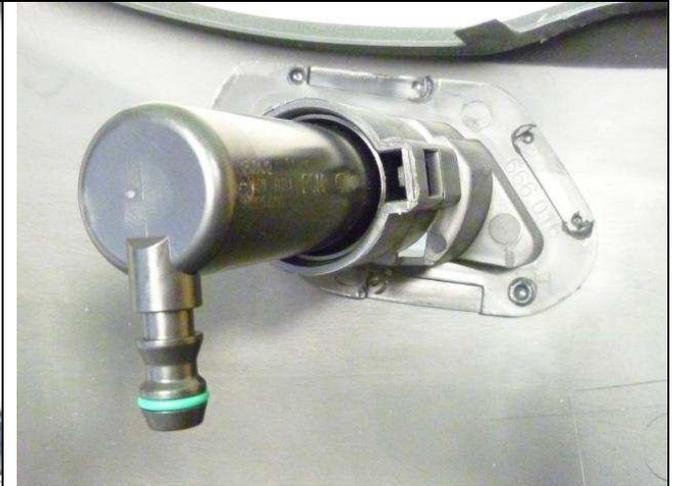
A close-up photograph of the tested product charging port. It is identical in design to the original equipment, but the green ring at the base of the black cylindrical connector is a different shade of green. |
