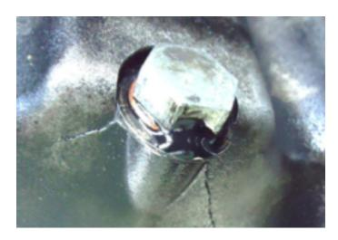
Example of **over-tightening** the oil drain bolt causing the crack of the oil pan because it is made in aluminum and leaving it totally unusable.
