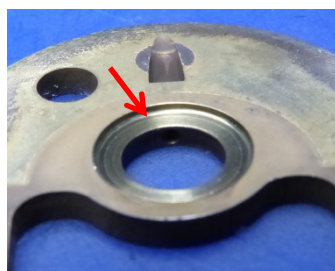
Axial bearing worn by axial thrust
