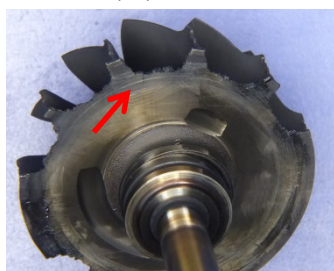
turbine wheel – grazed on housing
