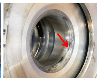
abraded compressor housing
