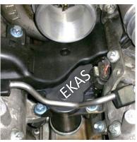
Oil accumulation in the intake duct of the turbocharger always originate from the crankcase ventilation. Check if the crankcase ventilation is working correctly and check the inner crankcase pressure. Use our BTS tool **MESS01** to do so.
