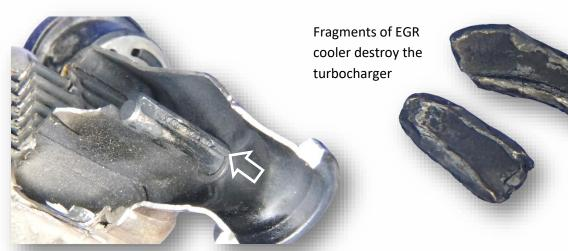
Cut-open EGR cooler with broken control flap
