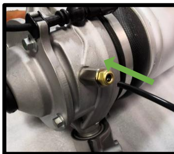
2、 Slide the threaded Part along the pipe path
