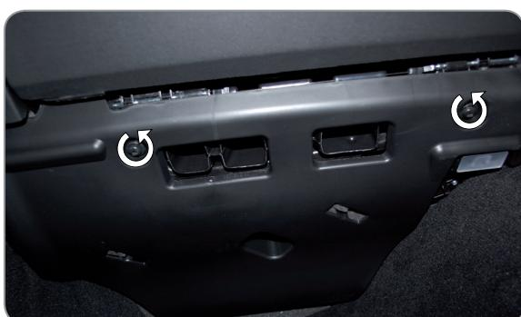
(EN) Loosen the screws that hold the shields of the filter chamber cover
