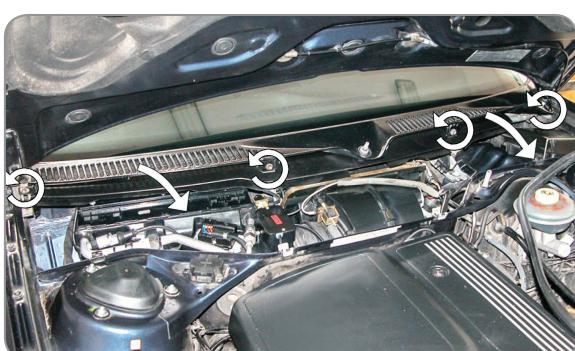
EN) Loosen the screws of the cover under the windshield. Remove the segment of the screen under the windshield
