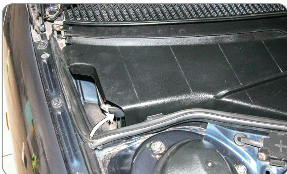
EN) Remove the rubber seal
