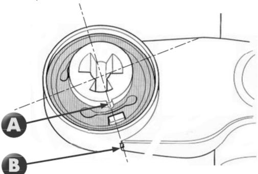
The identification mark on the face of the bush (A) must be aligned with the edge of the trailing arm on the axle beam (B)
