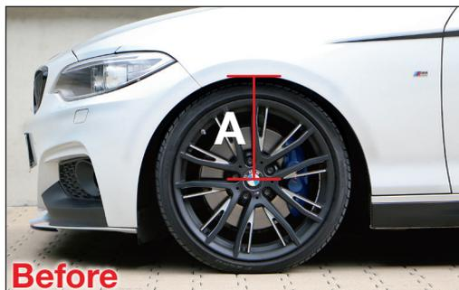
Measurement A: Wheel hub centre – fender edge
