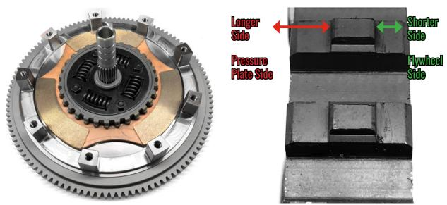
7. Fit the first intermediate plate onto the flywheel assembly, followed by the second ceramic lining.
