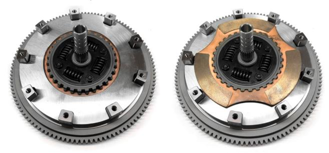
8. Fit the upper casting to the flywheel assembly, making sure that the flat friction surface is against the ceramic facing.
