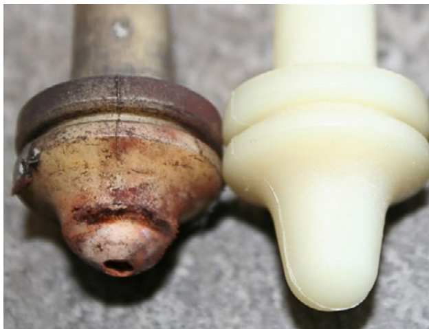
Example of a used OEM plastic pivot ball (left) & a new OEM plastic pivot ball (right) for the same application.
