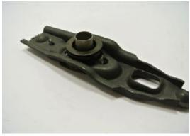
2) Remove bearing and carrier from the replacement snout. Rotate the snout to align the tabs/grooves in the snout/ carrier to slide them apart.
