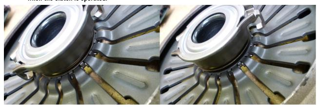
2. To remove the bearing from the cover a wedge will need to be used between the bearing and the bearing locating collar (a screwdriver can be used for this). Carefully twist the wedge so the bearing is removed on a slight angle. Removing the bearing on this angle will assist in the snap ring becoming dislodged from the locating groove.
