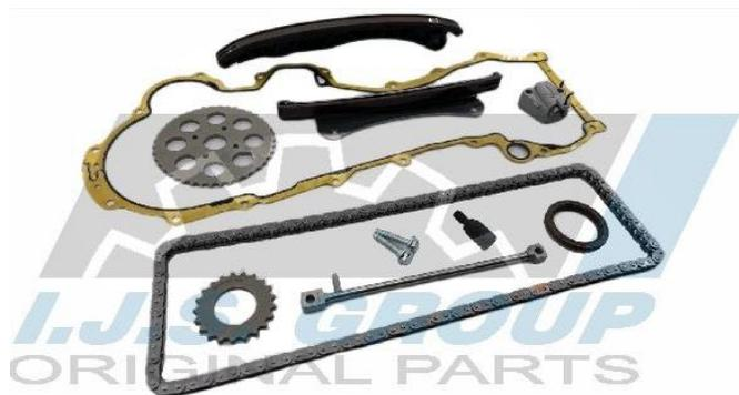
The kit now contains the latest generation EURO 6 Stop/Start timing chain which is made from modified materials and has pierced rollers, improving oil flow to the internal pins & rollers.
