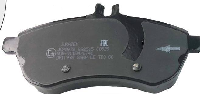
Fitting directional pads the wrong way may result in brake judder and ultimately high pitch squeal.
