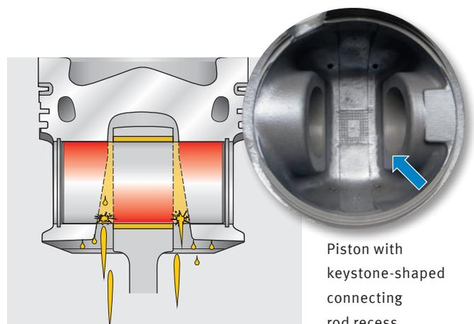
Piston with keystone-shaped connecting rod recess
