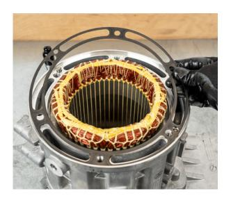
• If present: Remove the spring washer from the lower bearing seat
