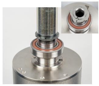
• Press the bearing with the housing cover onto the rotor
