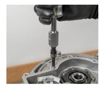
• Remove the high-voltage connections of the stator from the high-voltage terminal
