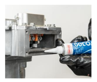
• Mount the upper cover and tighten the bolts to 11 Nm
