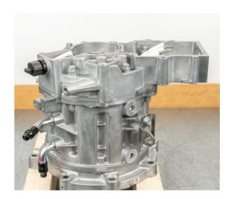
Mount the high-voltage terminal and tighten it to 10 Nm
