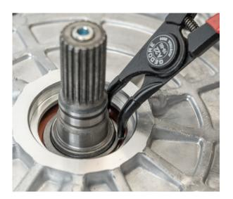
• Install the new sealing ring on the rotor shaft
