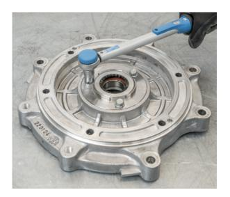
• Remove the bearing, rotor position sensor encoder, and snap ring from the rotor shaft
