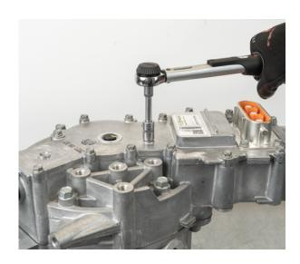
• Mount the bolts of the high-voltage connection and tighten to 10 Nm
