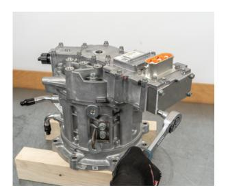
• Remove the bolts of the high-voltage connection
