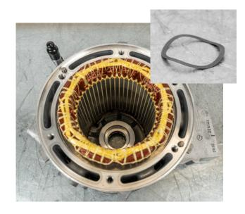
• Turn the stator housing over and support it at the housing
