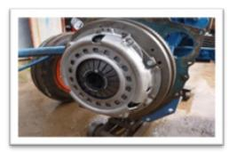
If the flywheel face has a glazed or polished appearance this indicates that repeated heating and cooling during the life of the previous clutch has created a hard skin. It is recommended that this be removed by grinding.
