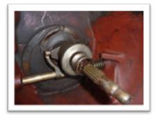
Clutch pedal free play set to a minimum of 30 – 50mm. The Pedal height can also be set to a comfortable operating position. Adjustments to both are made at the clevis on the clutch control rod.
