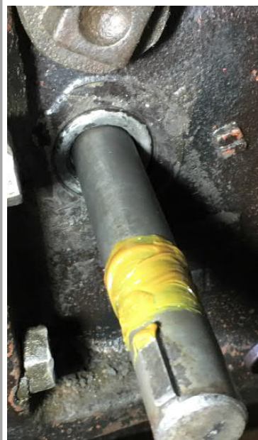
Step 16 – Fit new shaft and lubricate
