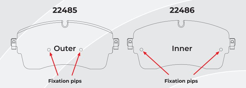
Due to these different locations of the pips, the parts are not interchangeable in the caliper. WVA 22485 is for the outer side, 22486 is for the inner side. Swapping the sides of these parts would cause the piston or respectively the fingers of the caliper to push against the pips. This could result in noise issues or an uneven wear of the friction material. Therefore, please look at the brake pads carefully to ensure that they are not mixed up prior to assembly.
