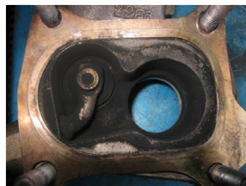
Gasket incorrectly mounted
