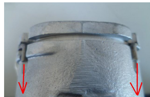
Both tips are facing the same direction
