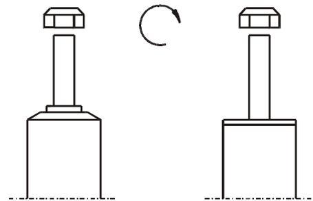
Do not use an impact tool to loosen or tighten fasteners due to possible damage to the product. Self-locking nuts must only be used once!
