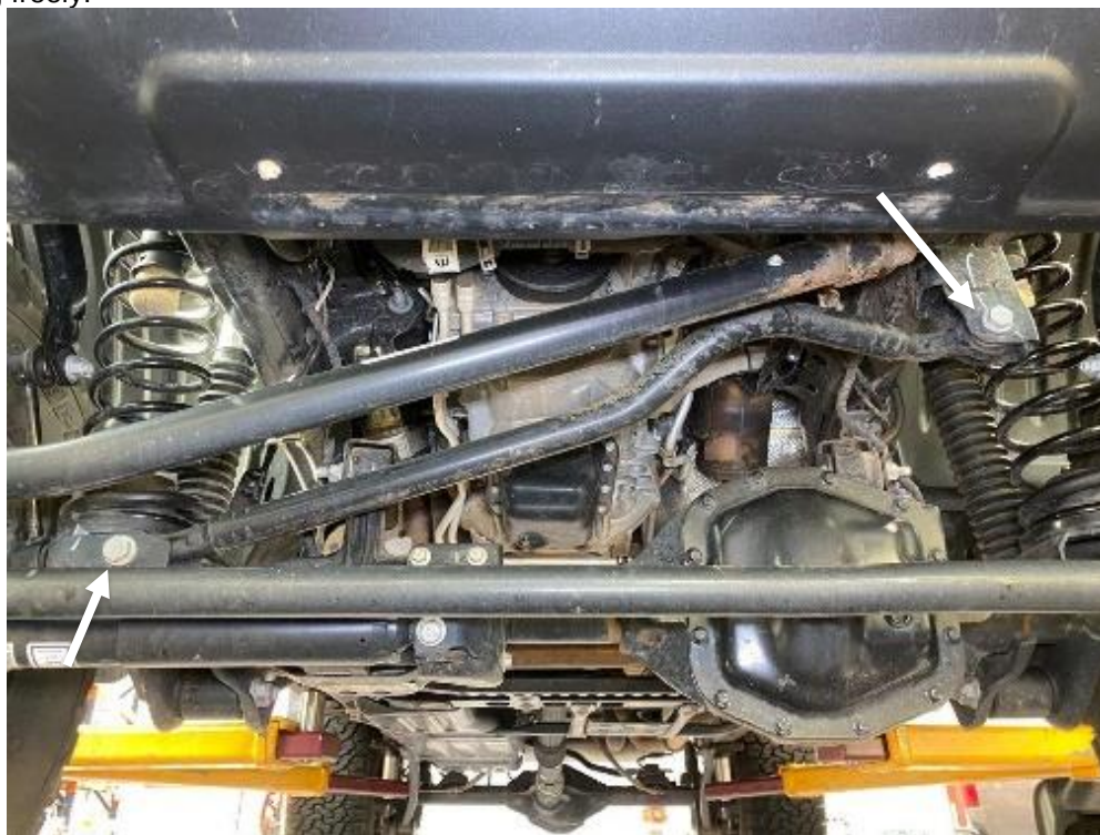
Track Bar Bolts
