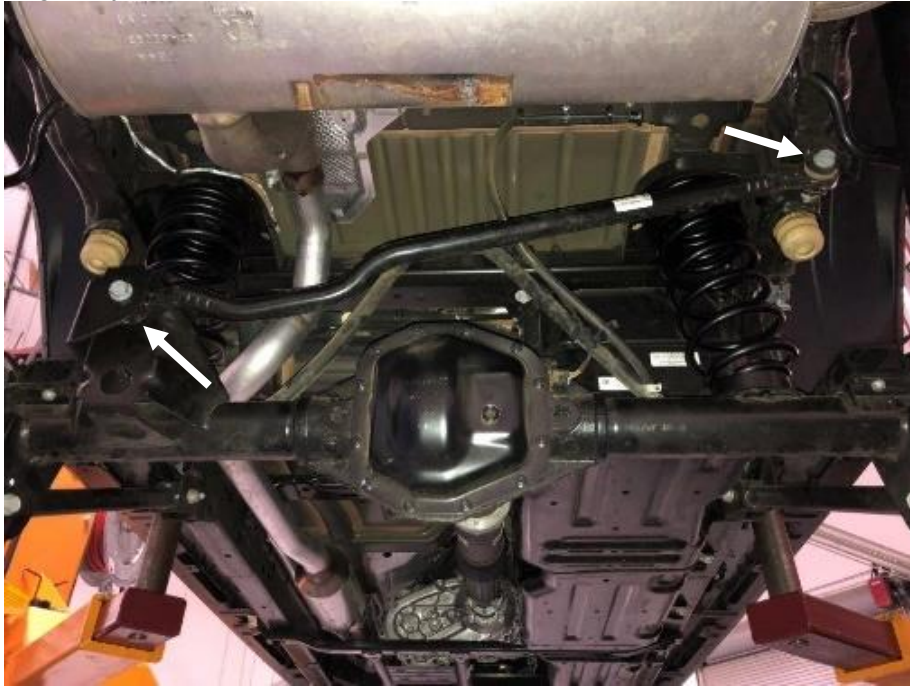
Track Bar Bolts
