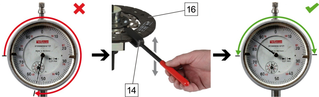
Fig. 10: Aligning clutch disk
