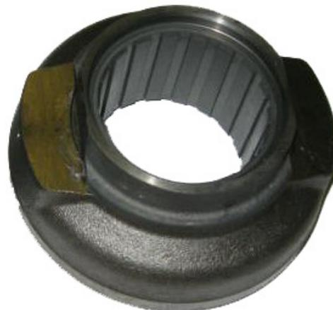
Fig. 4: Releaser with plastic slide sleeve
