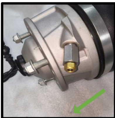
1.Remove and dispose of shipping pins
