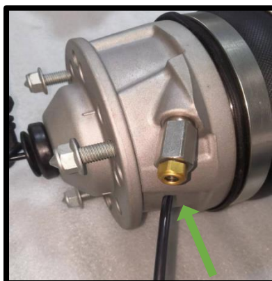
2.Insert the air line into the connector and press until it is felt to engage
