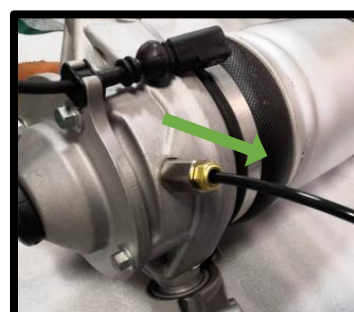
4. Remove the threaded part, disassembly is complete
