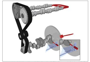
Image 1: Timing belt drive with camshaft locking plate (red) in place, camshaft timing pin (red) and flywheel locking tool (red)
