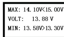
The actual test voltage is 13.88 V, the standard maximum voltage is 15.00 V (with 24 V system the standard maximum voltage is 30.00 V), the tested maximum voltage is 14.10 V. The other value indicates that the actual test voltage is 13.88 V, the standard minimum voltage is 13.30 V (for the 24 V system the standard minimum voltage is 26.60 V), the tested minimum voltage is 13.58 V.
