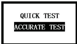
(5) Press the <▲><▼> button to select the test standard according to the standard of the battery. If it is the JIS standard, you must check the CCA value against the comparison table. Then select CCA (SAE) as the test standard and press <ENTER>. See figure:
