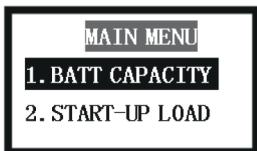
(3) Press the <▲><▼> button to select the type of battery. Then press <ENTER>. See figure:
