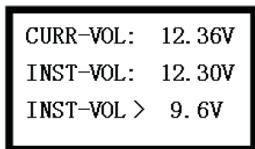
As shown in the image, the current test voltage is 12.36 V, the standard voltage is 9.6 V (in a 24 V system the standard voltage is 16 V), and the lowest voltage is 12.30 V.
