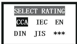
(6) According to the label on the battery, press the button <▲><▼> to set the nominal value. See image:
