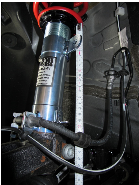
Pic 1: FA spring plate adjustment dimension (Picture may vary)
