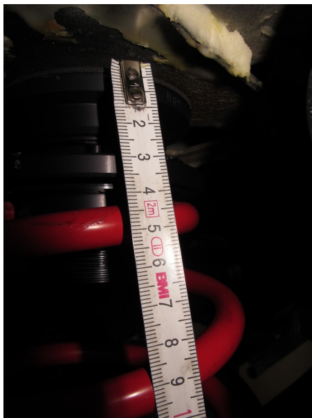
Pic 2: RA spring plate adjustment dimension (Picture may vary)
