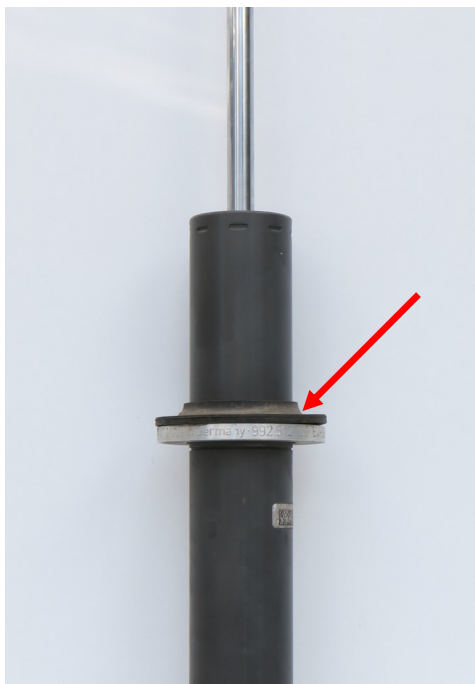
Abb. 4: Federteller demontieren Fig. 4: Dismantle the spring plate
