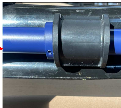
Fig. 2: Mounting of the Anti-Roll Bar ends
