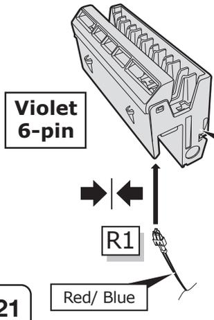
Locate 1 unoccupied fuse plug-in positions (B+/30)!
