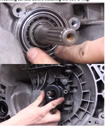
Carefully install the new concentric slave cylinder and reinstall the 3 mounting bolts.
