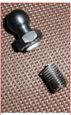
Pivot balls can become shorter or completely shear as a result of wear. Carefully check for any damage.
