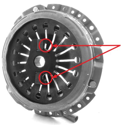
Clutch Fork goes in from this side. Ensure the circled areas are facing the clutch fork before installing the gearbox.
