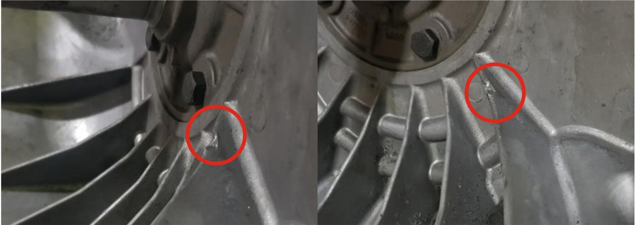
To allow for maximum fork movement and clutch wear, ACS recommends making a modification to the bellhousing ribs by grinding away a small section to avoid contact with the fork as shown in the below photos. Remove any sharp edges and burrs and test fit the fork prior to reinstallation of the clutch.
