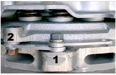
**Bolt 1: Long Bolt Spring Washer** Thin Washer Straps X 4 Thick Washer Straps X 5 **Thick Washer** Shim Washer
