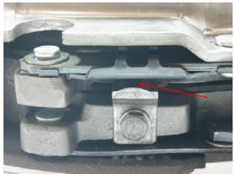
As shown the Hammer Centralizers are not set and have a gap between the centralizer and the strap landing.
