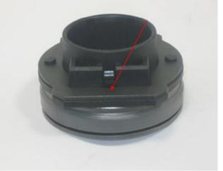
The release bearing in this kit is flat where the bearing fits to the release fork.
