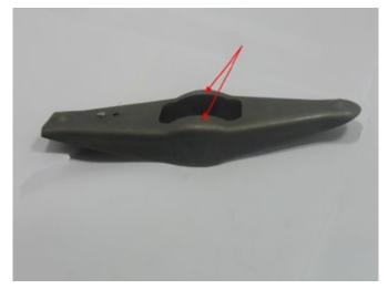
The fork that suits the release bearing in this kit should be raised where the release bearing pivots.
