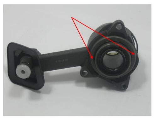
If the sealer is not added, gearbox oil could leak and contaminate the clutch causing it to slip. Once the clutch has been contaminated with this type of oil the clutch would need to be replaced.
