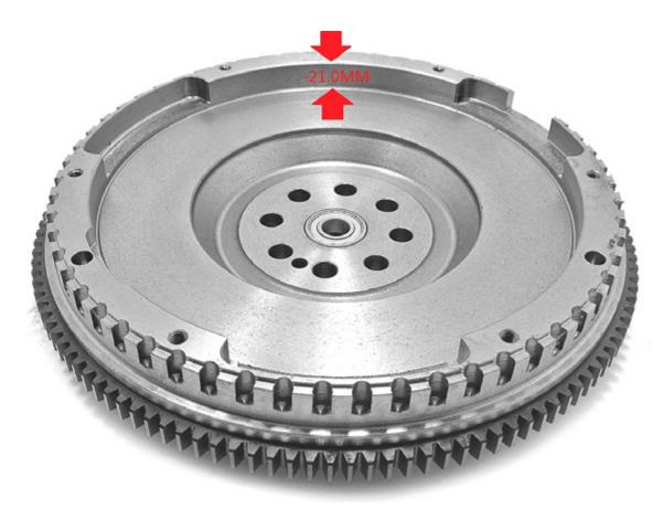
It has also been identified that there are 2 different bearing bore diameters based on the kit brand
