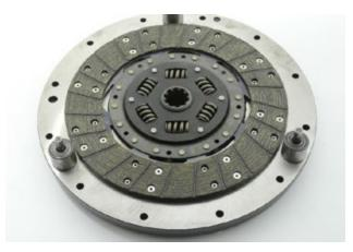
Fit second clutch disc. Closely note direction of hub and clutch disc used. 'Gearbox Side' sticker faces pressure plate.
