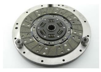
Flywheel side clutch disc fitted in direction shown. Closely note direction of hub and disc used. 'Engine Side' sticker faces Flywheel
