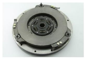
Fit intermediate plate. Note direction of release straps.
