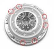
The diaphragm conversion cover (CFD28103) uses the holes marked. This cover suits the single drill flywheel. The clutch cover whilst has 9 bolts holes only 6 are use (3 mounting holes -smaller diameterand 3 clamping holes-larger diameter) if required the extra holes can be used but the flywheel will need the holes drilled and tapped.
