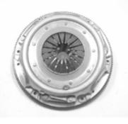
This clutch cover (CFD28102) suits the multi drilled Ford flywheel. The Ford multi drilled flywheel has been designed and drilled to suit various Ford cover stampings. If this cover is used on the Ford single drilled flywheel only 3 mounting holes will locate the cover and the other 3 will need to be drilled and tapped.
