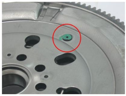
With these shipping pins it will not be possible to check for free play when the flywheel is new. These shipping pins do not need to be removed upon installation and will sheer off automatically during operation.
